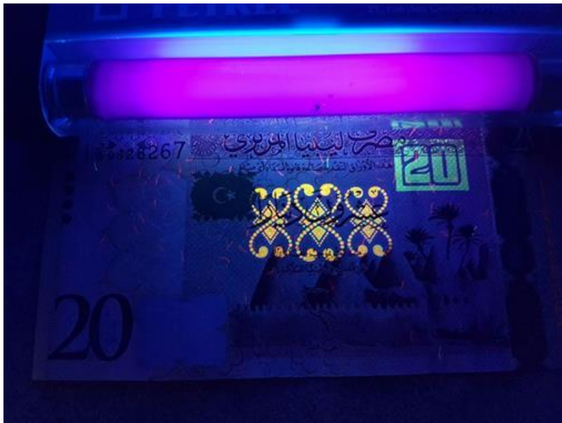
Photo 6: Covert features on front of original banknote
