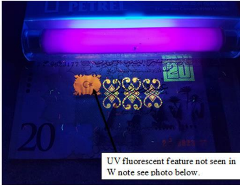
Photo 5: UV features on front of alternative banknote
